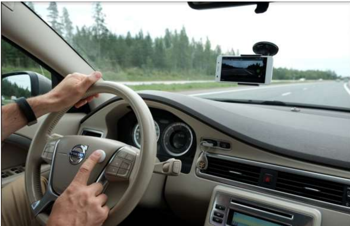
Figure 1: Mobile phone and annotation tool for capturing video from moving vehicles
