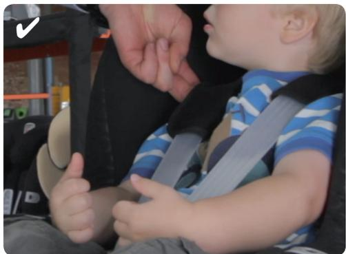
The tension of your child's harness is correct when you can place two fingers between the strap and the child's shoulder.
