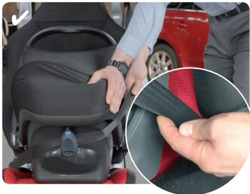
The seatbelt must be routed properly before tightening. Push down on the seat and pull the belt through to remove the slack and help tighten. Flick the belt at the beginning to check the tension; it should be tight.
