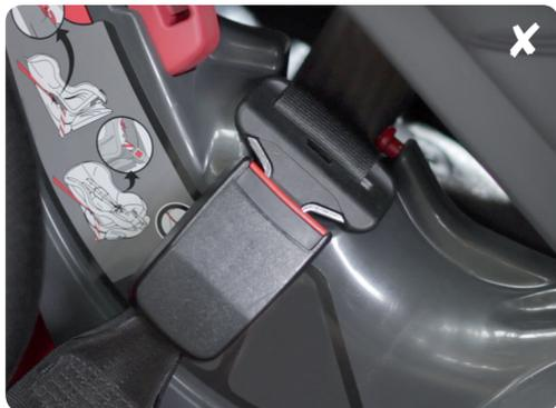
Buckle crunch is caused when the buckle is bent over the side of the child seat. The correct position for the buckle is straight, located just below the side of the child seat.
